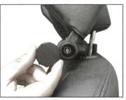
3.Install the left and right wings on both ends of the headrest bracket and tighten the plastic screw cap.
